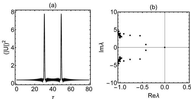
FIG. 5. A stable bound state of two dissipative solitons corresponding to a black point in Fig. 4,  $\delta = 0.02$ . (a) Intensity distribution and (b) eigenvalue spectrum. Other parameter values are the same as for Fig. 4.
