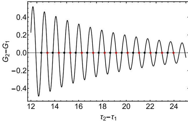
FIG. 4. Right-hand side of Eq. (16) as a function of the soliton separation  $\tau_2 - \tau_1$ . Black (red) dots indicate the separations of the two solitons in stable (unstable) bound states calculated numerically. Parameter values:  $S = 2.0$ ,  $\theta = 3.5$ ,  $\delta = 0.02$ , and  $\beta_4 = 0.025$ .
