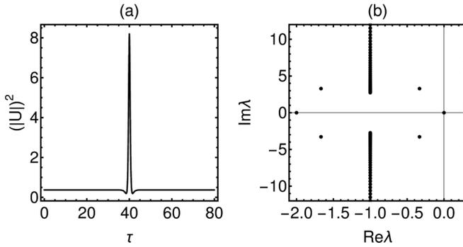
FIG. 2. (a) Soliton solution of the Lugiato-Lefever equation (1) with  $\beta_3 = \beta_4 = \delta = 0$  and (b) eigenvalue spectrum obtained by numerical linear stability analysis of this solution. Other parameters are the same as in Fig. 1.
