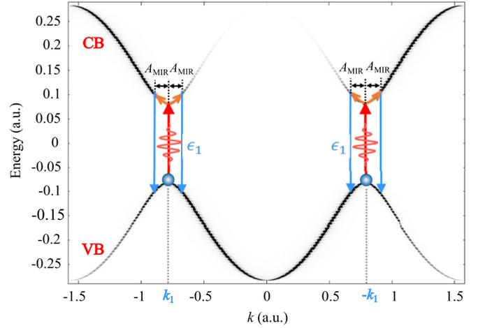
FIG. 2. Illustration of electron dynamics with only MIR driving field. The electrons are promoted via tunnel channels.
