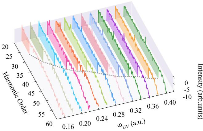
FIG. 5. The harmonic spectra in the cases of  $\omega_{UV}$  varying from 0.16 to 0.40 a.u. with a step of 0.2 a.u.
