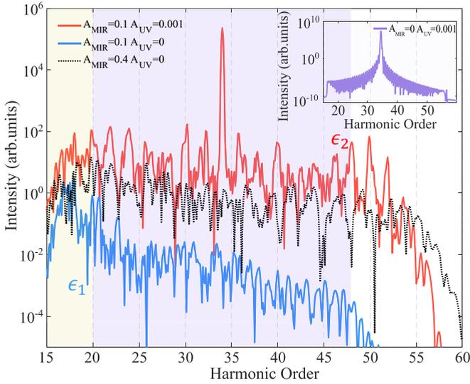
FIG. 1. The harmonic spectra in the cases of  $A_{\text{MIR}} = 0.1$  a.u.,  $A_{\text{UV}} = 0.001$  a.u.;  $A_{\text{MIR}} = 0.1$  a.u.,  $A_{\text{UV}} = 0$ ; and  $A_{\text{MIR}} = 0.4$  a.u.,  $A_{\text{UV}} = 0$ . The harmonic spectra have been shifted vertically for comparison. The harmonic spectrum in the case with pure UV light (see the violet solid line) is presented in the inset.
