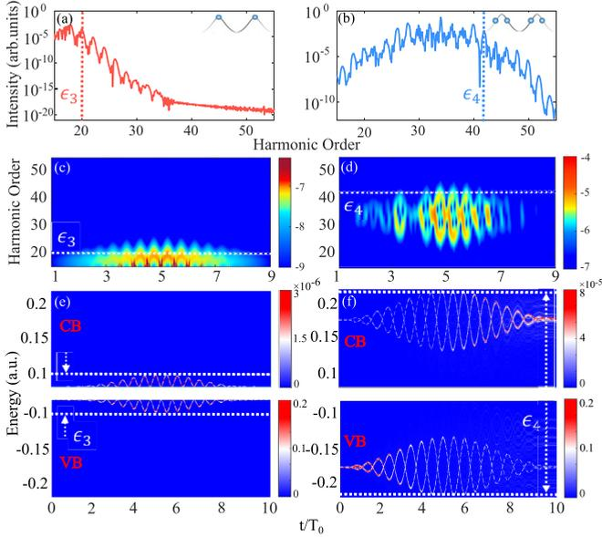
FIG. 4. Comparison of the cases without (left column) and with (right column) the UV field considering only electrons with typical initial crystal momenta. [(a), (b)] The harmonic spectra without and with the UV field. [(c), (d)] The time-frequency analysis of the HHG without and with the UV field. [(e), (f)] The TDPI and the semiclassical trajectories in the reciprocal space without and with the UV field.
