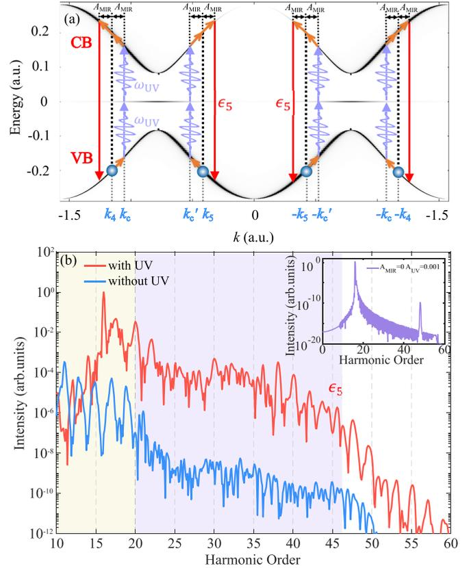
FIG. 6. (a) Illustration of the electron dynamics with the UV field ( $\omega_{UV} = 0.16$  a.u.) in the topological semiconductor. (b) The harmonic spectra with and without the UV field in the topological semiconductor. The harmonic spectrum in the case with pure UV light (see the violet solid line) is presented in the inset.
