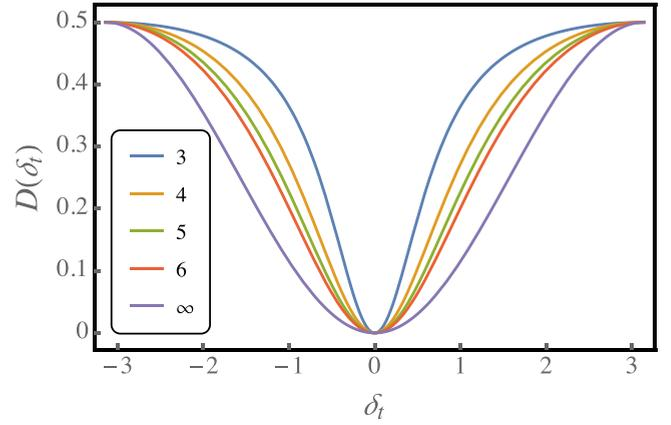
FIG. 4. Relation between distance  $D(\delta_t)$  and uncertainty of time  $\delta_t$  for different dimensions (represented by different colors). Here, we assume  $\sum_{\mu, \nu \neq \mu}^{0, \dots, d-1} |\mathcal{S}_{\mu\nu}|^2 = 1$ .
