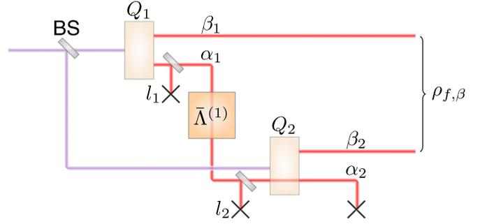
FIG. 3. LWM interferometer with loss. Two BS are placed in mode 1 of source  $Q_1$  before and after transformation.
