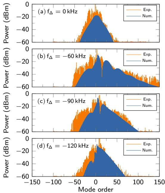
FIG. 4. Experimental and numerical spectra for various values of the frequency mismatch  $f_{\Delta}$ . The parameters for the numerical simulations were  $\alpha = 0$  and  $\beta = -0.008$ . The input pulse was a Gaussian with a 4.2 ps pulse width.
