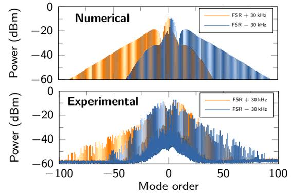
FIG. 3. Kerr comb spectra at the output of the WGM resonator for a repetition rate mismatch of  $\pm 30$  kHz relative to the FSR. Top: Numerical simulation using Eq. (9) with parameter  $\alpha = 0$ ,  $F = 8$ ,  $\beta = -0.005$ , and considering a Gaussian pulse with a 4.2 ps width. Bottom: Experimental spectra using the experimental setup presented in Fig. 1.
