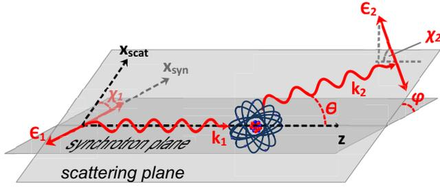
FIG. 1. The geometry of Rayleigh scattering. The propagation direction of the incident light is chosen as the  $z$  axis. Together with the incident linear polarization vector  $\epsilon_1$ , the  $z$  axis defines the synchrotron plane. For the theoretical description, the plane, spanned by the propagation directions of incident and outgoing photons, is important. This plane is usually referred to as the scattering plane.
