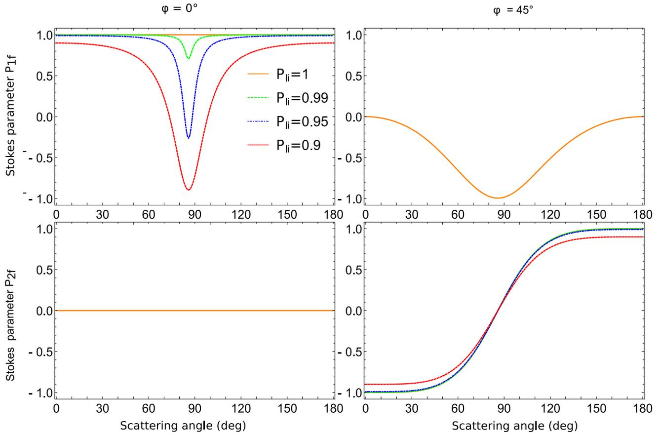
FIG. 2. The Stokes parameters of the scattered radiation  $P_{1f}$  and  $P_{2f}$  depending on the scattering angle  $\theta$ , for different degrees of linear polarization of the incoming radiation  $P_{ii}$  and different azimuthal angles  $\varphi$  for scattering of 145 keV x rays off a lead atom (Pb,  $Z = 82$ ). The results of  $P_{1f}(\varphi = 45^\circ)$  and  $P_{2f}(\varphi = 0^\circ)$  for different initial depolarizations coincide as predicted by Eqs. (17) and (18).
