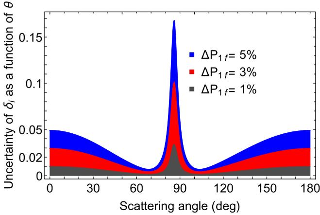
FIG. 3. Initial depolarization  $\delta_i = 0.02$  determined through theoretical calculations of  $P_{1f}(\varphi = 0^\circ)$  and  $P_{1f}(\varphi = 45^\circ)$  with initial photon energy of 145 keV scattered by a lead atom. The gray, red, and blue shadowed areas show the angular-dependent uncertainty in the determination of  $\delta_i$  for a relative uncertainty of 1%, 3%, and 5% in the measurements of  $P_{1f}$ .
