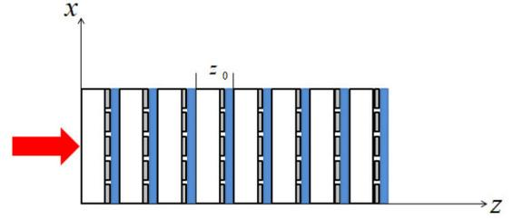
FIG. 3. Schematic illustration of our proposed optical system with multilayer media, where the blue layers denote Kerr media and the gray layers represent the phase gratings.
