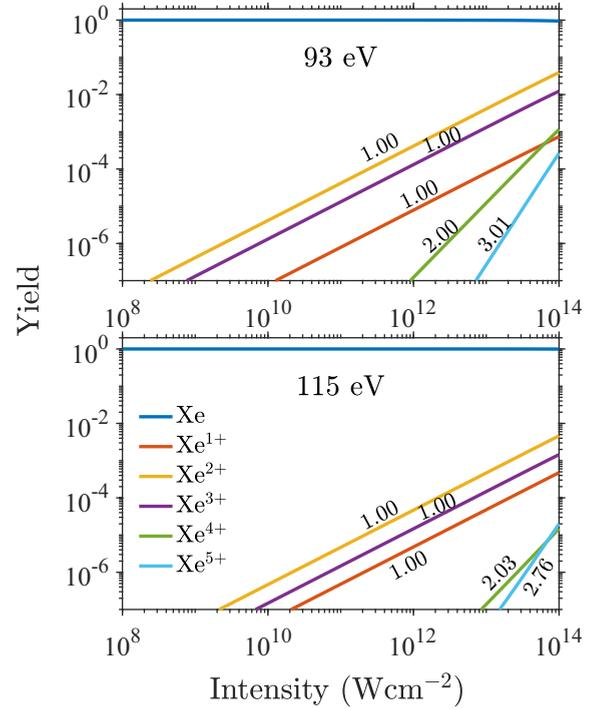
FIG. 3. Log-log plot of the ion yields versus pulse intensity for the 93 eV pulse (a) and for the 115 eV pulse (b). The numbers along the lines correspond to the slope of each of the yields versus intensity.
