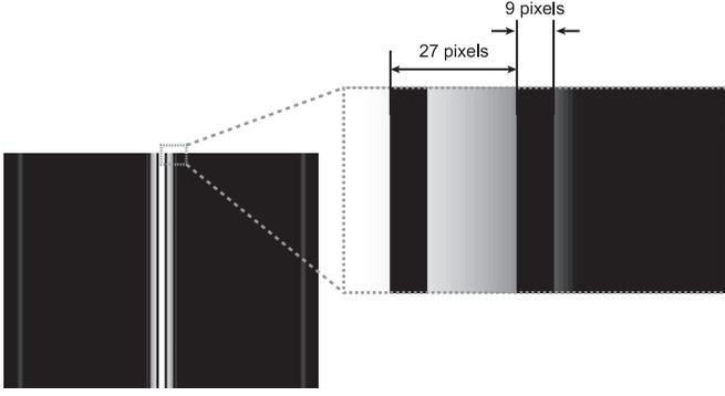
FIG. 2. Simulation the non-Markovian noise on the DMD screen [the experimental results are shown in Fig. 3(e)]. The enlarged image (right) highlights the periodic attributes. The grating constant ( $d = 27$  pixels) and the width of each seam ( $a = 18$  pixels) are clearly discernible. Here, 1 pixel =  $13.7 \mu\text{m}$ .
