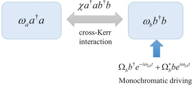
FIG. 1. Schematic diagram of the system. Two bosonic modes ( $a$  and  $b$ ) with resonance frequencies  $\omega_a$  and  $\omega_b$  are coupled with each other by a cross-Kerr interaction with coupling strength  $\chi$ . One of the modes (e.g., mode  $b$ ) is driven by a monochromatic field with the driving frequency  $\omega_{Lb}$  and driving amplitude  $\Omega_b$ .
