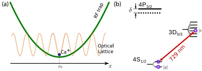
FIG. 1. (a) Optical lattice and harmonic trapping potential; (b) electronic level scheme for  $^{40}\text{Ca}^+$ . The phase of the OL is stabilized so that one of its minima coincides with the minimum of the trapping potential. The OL has  $\lambda_{\text{OL}} = 854$  nm and is visible only when the ion is in state  $|e\rangle$ . State-dependent squeezing is induced by modulation of the intensity of the OL.
