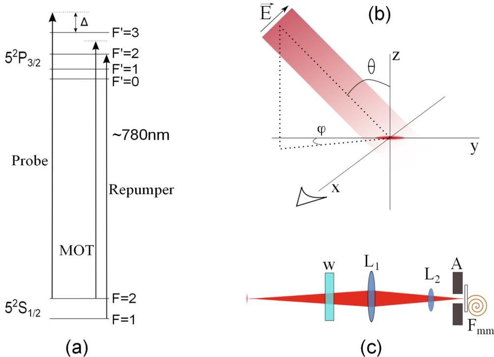
FIG. 1. Basic experimental scheme. (a) Relevant  $^{87}\text{Rb}$  energy levels. (b) Geometry of probe optical excitation and fluorescence collection. The angles  $\theta = 23^\circ$  and  $\phi = 30^\circ$ . (c) Fluorescence detection arm, viewing down the  $x$  axis. Light is detected in the far field through a window (w) and focused into a  $600\ \mu\text{m}$  diameter multimode optical fiber  $F_{mm}$  with a pair of lenses  $L_1$  and  $L_2$  as shown.
