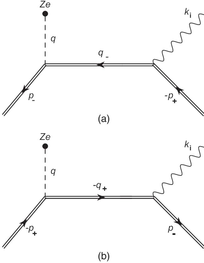
FIG. 1. Feynman diagrams of the PPP process on the nucleus in the field of a plane electromagnetic wave. Double incoming and outgoing lines correspond to the Volkov functions of the electron and positron in the initial and final states, the inner line corresponds to the Green's function of the fermion in the field of a plane wave (4). Wavy line corresponds to four-momentum of the initial gamma quantum. Dashed line stands for four-momentum of pseudophoton of recoil
