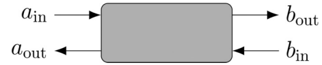
FIG. 2. Input and output fields coupled to a two-port black box quantum network. The input and output operators are continuous mode (as functions of frequency \omega ) annihilation operators, satisfying canonical commutation relations [32]. Here the mode a_{in}(\omega) carries the single photon input state, the reflected mode is described by a_{out}(\omega) , and the output mode b_{out}(\omega) contains the excitation energy if the input energy successfully traversed the network (and may serve as input to the next part of the photodetection process, e.g., amplification; see Ref. [12]). b_{in}(\omega) may contain thermal excitations, but is never occupied by the photon we wish to detect.
