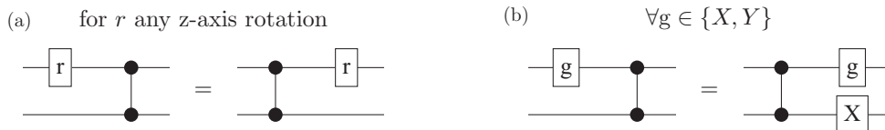
FIG. 6. Well-known cases where a one-qubit gate can be pushed through a CZ gate. In case (b) a by-product gate is created. These by-product gates can in turn be pushed through other CZs.
