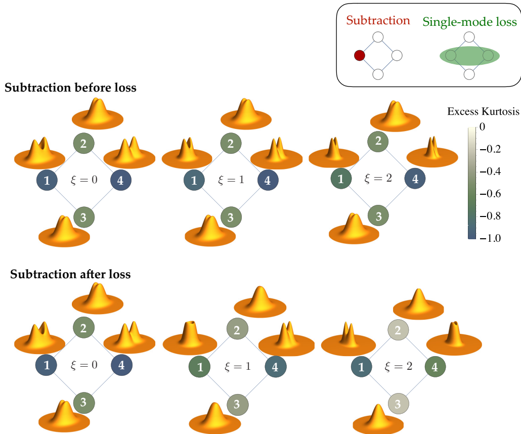
FIG. 8. Graph state (50) of four vertices (modes), with a photon subtracted in the mode associated with the red vertex (inset), probed for different degrees \xi of losses. The single-mode reduced Wigner function is shown for each vertex k . The minimal excess kurtosis (51) in each vertex is represented by the color code. Losses (53) act on a single mode that is a superposition of several vertices, as indicated in the inset (see main text for details). Losses and photon subtraction do not commute, hence we show both scenarios: subtraction prior to losses (top) and losses prior to subtraction (bottom). All modes in the initial squeezed vacuum V_0 are equally squeezed (i.e., s_1 = \dots = s_m ) at 10 dB.
