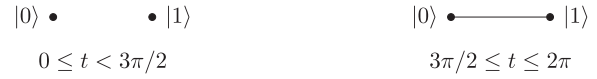
FIG. 5. A dynamic graph representation of the X gate consists of two graphs and the associated propagation times. This sequence of CTQW executes the logical bit flip operation on the graph state.
