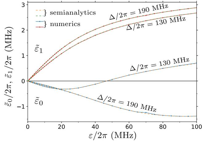
FIG. 6. Effective drive amplitudes  $\tilde{\epsilon}_0$  and  $\tilde{\epsilon}_1$  as functions of  $\epsilon$ , calculated numerically (solid lines with symbols) and using the semianalytical approach (26)–(29) (dashed lines, practically coinciding with the solid lines). We used  $g/2\pi = 3$  MHz,  $\eta_c/2\pi = \eta_c/2\pi = 300$  MHz, and two values for the detuning:  $\Delta/2\pi = 130$  and 190 MHz.
