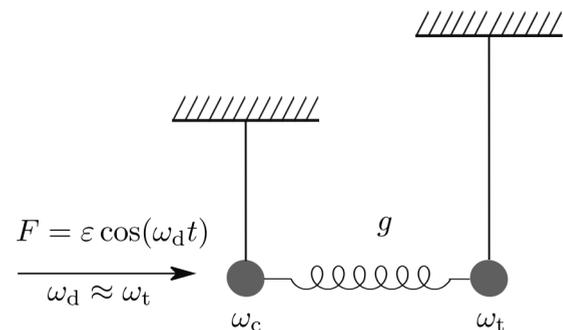
FIG. 2. Classical CR gate counterpart: two coupled nonlinear oscillators, with one oscillator driven by a periodic force  $F$  off-resonance with the other oscillator.
