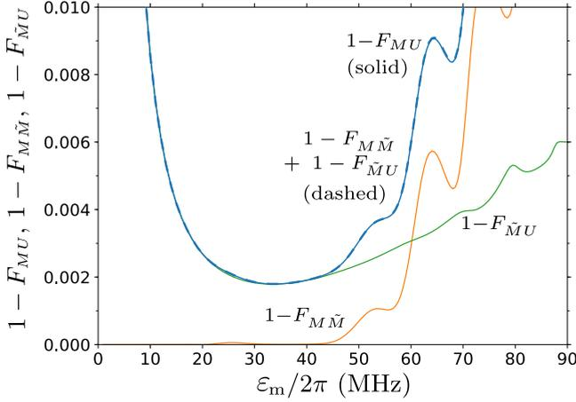
FIG. 15. Decomposition of the CNOT gate infidelity  $1 - F_{MU}$  (solid blue line) into the leakage contribution  $1 - F_{M\bar{M}}$  (orange line) and contribution  $1 - F_{\bar{M}U}$  due to imperfect unitaries (green line). The sum  $(1 - F_{M\bar{M}}) + (1 - F_{\bar{M}U})$  (dashed blue line) is practically indistinguishable from the solid blue line. We use  $\Delta/2\pi = 130$  MHz and the parameters from Fig. 14.
