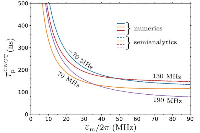
FIG. 10. CNOT gate duration  $\tau_p^{\text{CNOT}}$  (neglecting single-qubit rotations) as a function of the midpulse drive amplitude  $\varepsilon_m$  for several detunings:  $\Delta/2\pi = -70, 70, 130,$  and  $190$  MHz, while  $g/2\pi = 3$  MHz,  $\eta_c/2\pi = \eta_t/2\pi = 300$  MHz,  $\tau_r/\tau_p = 0.3$ , and  $\omega_d = \omega_t^{c0}$ . Solid lines are calculated numerically; dashed lines (almost coinciding with the solid lines) are calculated using the semianalytical method.
