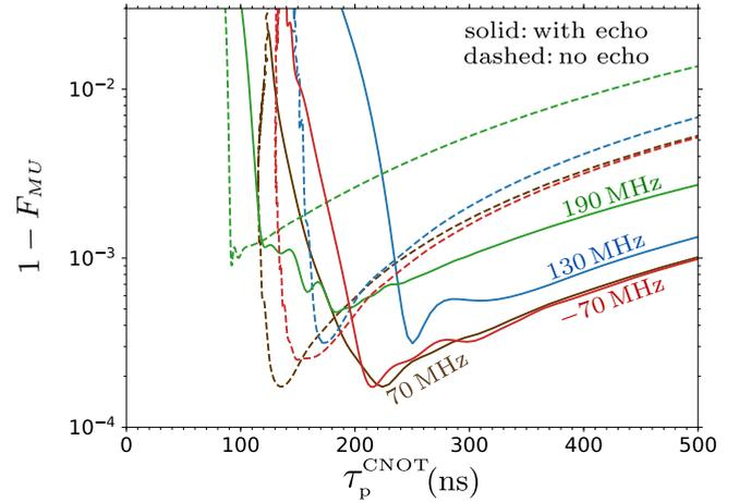
FIG. 23. CNOT gate infidelity  $1 - F_{MU}$  versus duration  $\tau_p^{\text{CNOT}}$  for the echo-CR gate (solid lines) and the basic CR gate (dashed lines). The detunings  $\Delta/2\pi$  are 190 MHz (green lines), 130 MHz (blue lines), 70 MHz (brown lines), and  $-70$  MHz (magenta lines). The parameters are the same as in Fig. 18, except we use  $\omega_d = (\omega_i^0 + \omega_i^1)/2$ . The lines are cut at the left for clarity.
