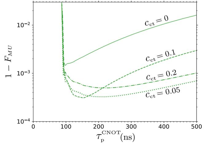
FIG. 22. CNOT gate infidelity  $1 - F_{MU}$  versus duration  $\tau_p^{\text{CNOT}}$  for  $\Delta/2\pi = 190$  MHz and several values of the microwave crosstalk coefficient:  $c_{ct} = 0$  (solid line),  $0.05$  (dotted line),  $0.1$  (dashed line), and  $0.2$  (dash-dotted line). The other parameters are the same as in Fig. 18. The lines are cut at the left for clarity.
