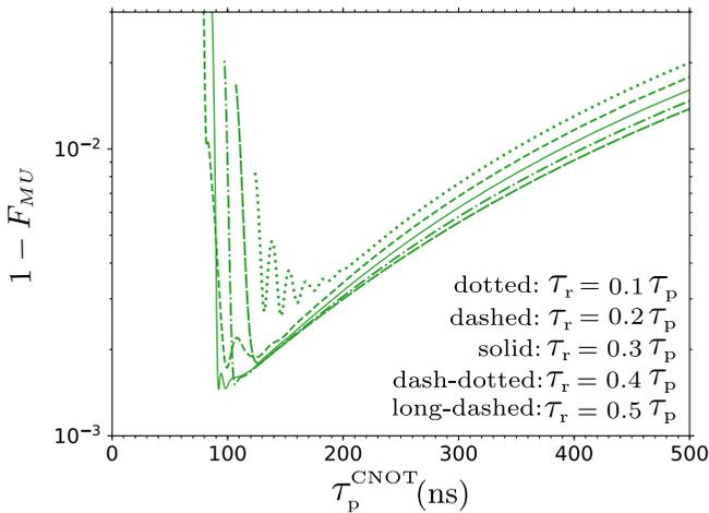
FIG. 21. CNOT gate infidelity  $1 - F_{MU}$  versus duration  $\tau_p^{\text{CNOT}}$  for  $\Delta/2\pi = 190$  MHz and several values of the relative duration of the pulse ramps:  $\tau_r/\tau_p = 0.1$  (dotted line),  $0.2$  (dashed line),  $0.3$  (solid line),  $0.4$  (dash-dotted line), and  $0.5$  (long-dashed line). The other parameters are the same as in Fig. 18. The lines are cut at the left for clarity.
