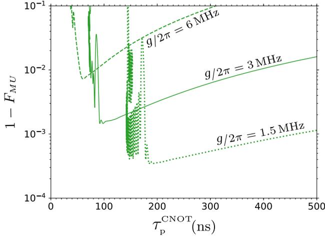
FIG. 20. CNOT gate infidelity  $1 - F_{MU}$  versus duration  $\tau_p^{\text{CNOT}}$  for  $\Delta/2\pi = 190$  MHz and several values of the qubit-qubit coupling:  $g/2\pi = 1.5, 3,$  and  $6$  MHz. The other parameters are the same as in Fig. 18.
