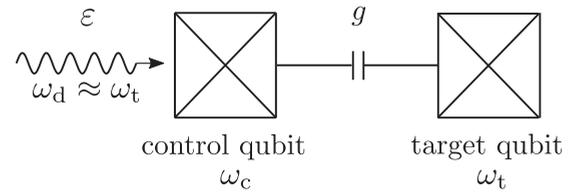
FIG. 1. Schematic of the CR gate. Detuned control and target qubits (transmons with frequencies  $\omega_c$  and  $\omega_t$ ) have coupling  $g$  and the control qubit is microwave driven at the frequency of the target qubit,  $\omega_d \approx \omega_t$ . The microwave drive amplitude is  $\epsilon$ .
