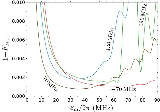
FIG. 14. Infidelity  $1 - F_{MU}$  of the CNOT-equivalent gate as a function of midpulse drive amplitude  $\varepsilon_m$  for several values of detuning:  $\Delta/2\pi = -70$  MHz (red line), 70 MHz (brown line), 130 MHz (blue line), and 190 MHz (green line). The other parameters are  $g/2\pi = 3$  MHz,  $\eta_c/2\pi = \eta_t/2\pi = 300$  MHz,  $\omega_d = \omega_t^{c0}$ , and  $\tau_r/\tau_p = 0.3$ .
