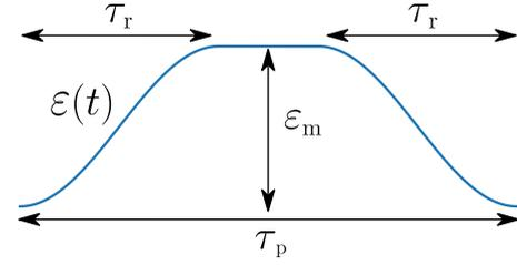
FIG. 9. Pulse shape  $\varepsilon(t)$  used in numerical simulations. The total pulse duration is  $\tau_p$ , each cosine-shaped ramp has duration  $\tau_r$ , and the drive amplitude in the middle flat part is  $\varepsilon_m$ .
