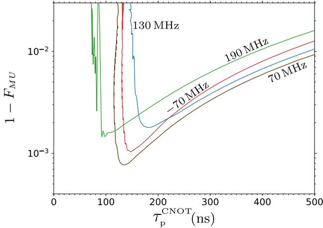
FIG. 18. Parametric plot for the CNOT gate infidelity  $1 - F_{MU}$  versus the CNOT gate duration  $\tau_p^{\text{CNOT}}$  (the running parameter is  $\varepsilon_m$ ) for the detunings  $\Delta/2\pi = -70, 70, 130,$  and  $190$  MHz. We assume  $g/2\pi = 3$  MHz,  $\eta_c/2\pi = \eta_t/2\pi = 300$  MHz,  $\omega_d = \omega_t^{c0}$ , and  $\tau_r/\tau_p = 0.3$ .
