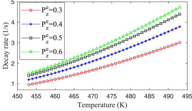
FIG. 8. Simulations of relationship between  $\lambda_{1r}$  and temperature as well as the polarization of Rb electrons  $P_z^e$ .
