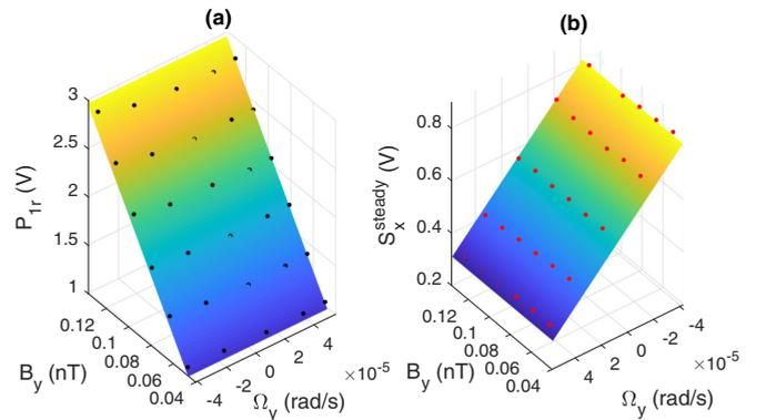
FIG. 7. The fitted  $P_{1r}$  and  $S_x^{\text{steady}}$  as functions of the angular velocity and magnetic field. The points represented in red and black are measurement points, and the colored planes are the fit to the data. The fitting functions of the subgraphs are  $P_{1r} = 21.86B_y - 0.0124$  and  $S_x^{\text{steady}} = -5124\Omega_y + 0.6048$ , respectively.
