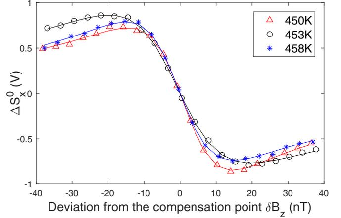
FIG. 4. The dependence of the difference between the initial and the steady state responses  $\Delta S_x^0$  on the deviation from the compensation point  $\delta B_z$  for different temperatures.
