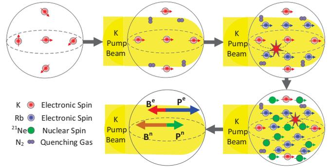
FIG. 1. Schematic of the polarization process and the simplified interaction model.
