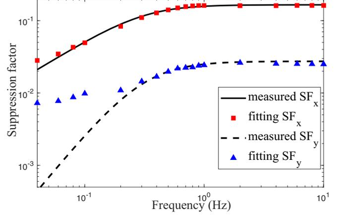
FIG. 9. Suppression of the comagnetometer response to oscillating fields along the X axis and the Y axis.
