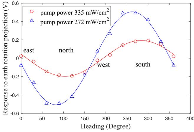
FIG. 5. The comagnetometer responses to the projection of earth rotation  $\Omega_y$ , with different pump power.
