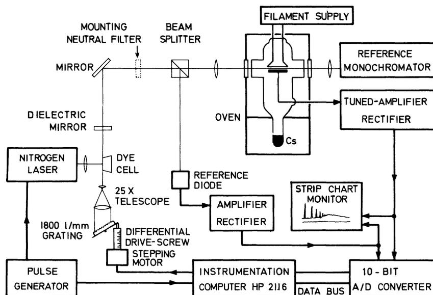
FIG. 2. Schematic representation of the arrangement of the tunable dye laser, cesium absorption cell with included detector diode, and data acquisition electronics used in these experiments.
