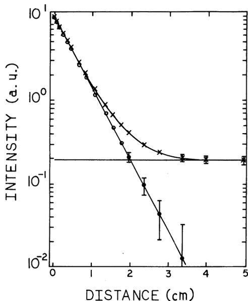
FIG. 7. Typical decay curve of the  $\bar{\lambda}=4114\text{-}\text{\AA}$  transition of F II. Intensity is in arbitrary units (a.u.). Beam energy was 25.2 keV. The lifetime for this decay curve was  $10.26 \pm 0.12$  ns.
