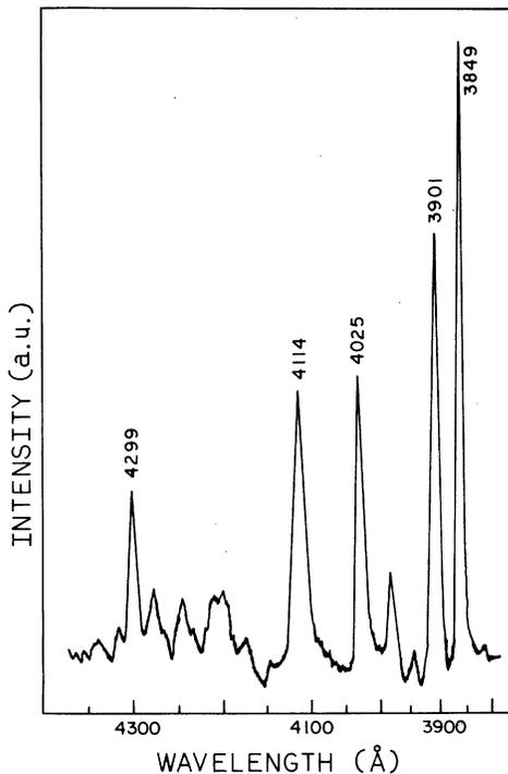
FIG. 5. Partial spectrum of an excited  $\text{HF}^+$  beam taken within the first 2 mm of the upstream end of the observation chamber. Intensity is in arbitrary units (a.u.).
