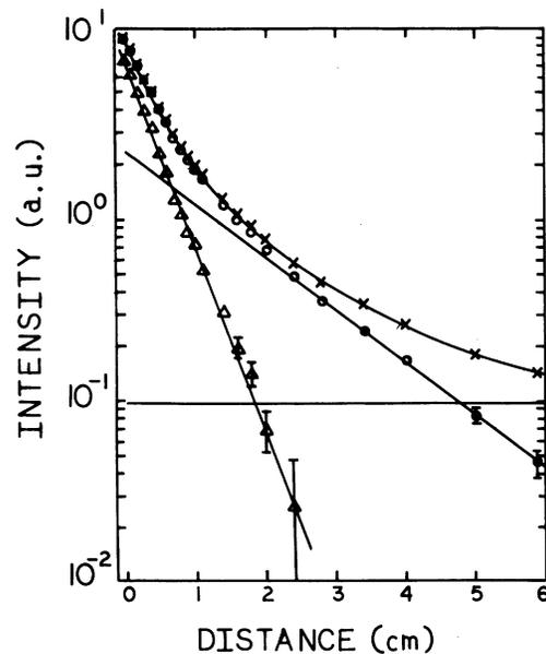
FIG. 6. Typical decay curve of the  $\bar{\lambda}=3849\text{-\AA}$  transition of F II. Intensity is in arbitrary units (a.u.) and is normalized to 10 at  $x=0$ . Beam energy was 25.2 keV. The lifetime for this decay curve was  $8.41 \pm 0.26 \text{ ns}$ .
