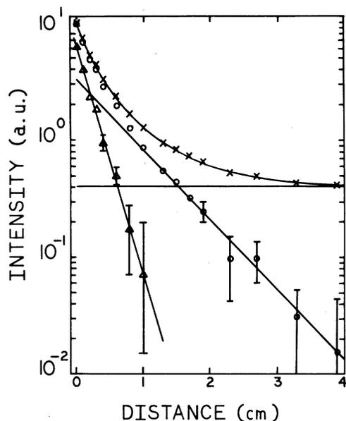
FIG. 8. Typical decay curve of the  $\bar{\lambda}=3602\text{-}\text{\AA}$  transition of F II. Intensity is in arbitrary units (a.u.). Beam energy was 26.0 keV. The lifetime for this decay curve was  $4.45 \pm 0.76$  ns.
