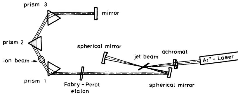
FIG. 3. Schematic drawing of the dye-laser resonator.
