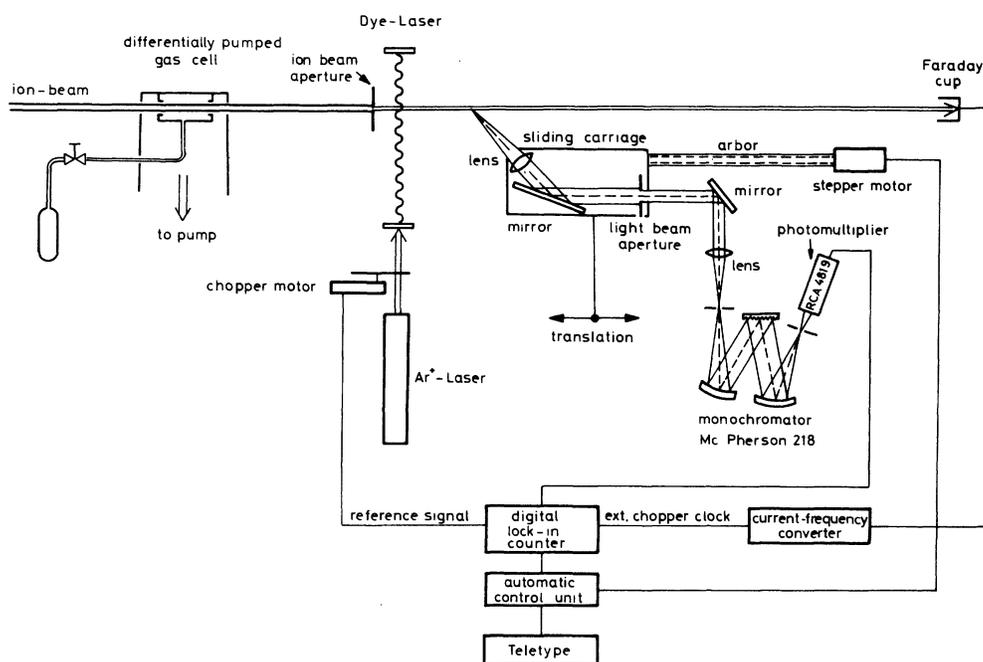
FIG. 2. Experimental arrangement of gas-laser excitation and following cascade-free lifetime measurement.
