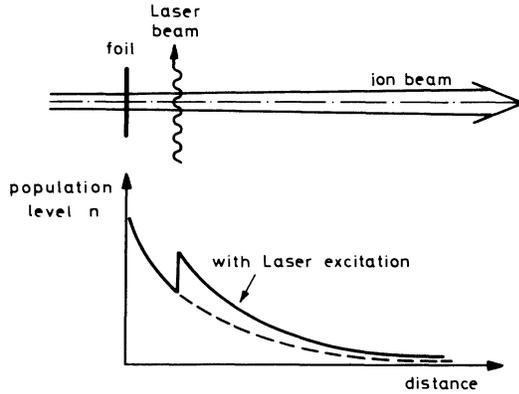
FIG. 1. Principal arrangement of foil-laser excitation and resulting population change of level  $n$  as a function of distance after the excitations.
