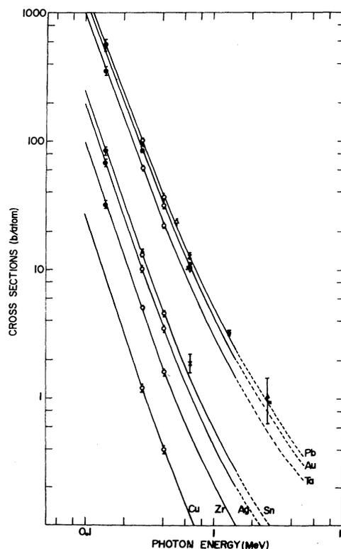
FIG. 4. Plot of  $K$ -shell photoelectric cross sections as functions of energy. ●, Ramakrishna Gowda and B. Sanjeevaiah (Ref. 8); ○, present work; X, Ghuman *et al.* (Ref. 6); Δ, Seeman (Ref. 2); ▽, DiLazzaro and Missoni (Ref. 5); ■, Bleeker *et al.* (Ref. 4); ▲, Davidson and Latyshev (Ref. 1) (the cross section for Pb as given in Ref. 9); — —, Scofield (Ref. 13); - - -, Schmickley and Pratt (Ref. 9).
