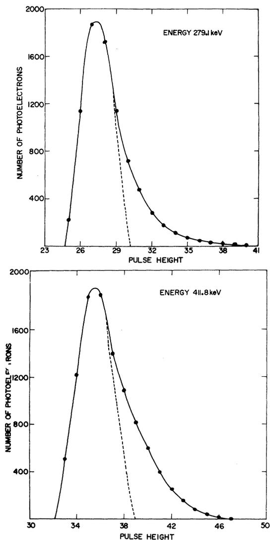
FIG. 3. Resolved photoelectron spectrum of lead (area under the Gaussian fitted to the spectrum gives the number of  $K$ -shell photoelectrons).
