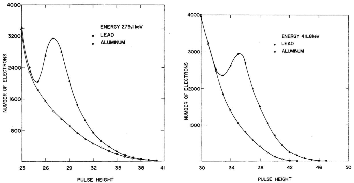
FIG. 2. Resolved electron spectra.
