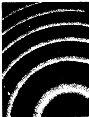
FIG. 2. Fabry-Perot interferogram of Stokes radiation showing two oscillating modes separated by \sim 0.3 \text{ cm}^{-1} . The inter-order spacing is \sim 3 \text{ cm}^{-1} .
