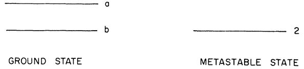
FIG. 3. Energy levels for and the notation for the model system using a two-level metastable atom with a two-level ground state.
