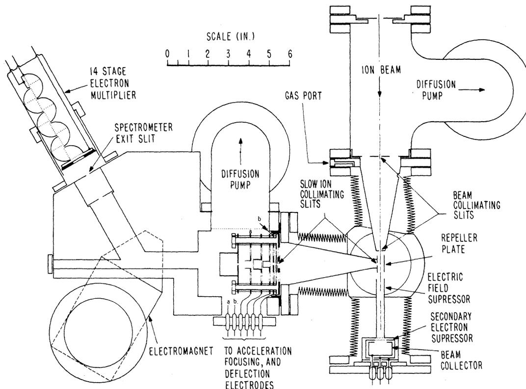
FIG. 1. Detailed drawing of collision and analysis regions.
