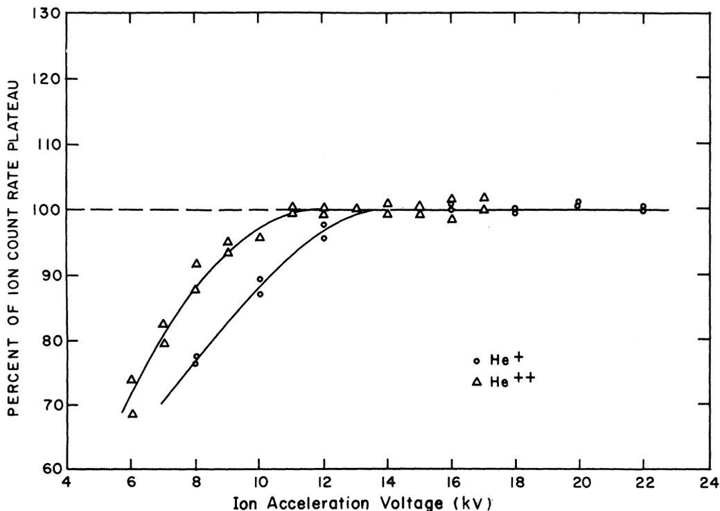
FIG. 2. Response of multiplier ion count rate to ion acceleration voltage.
