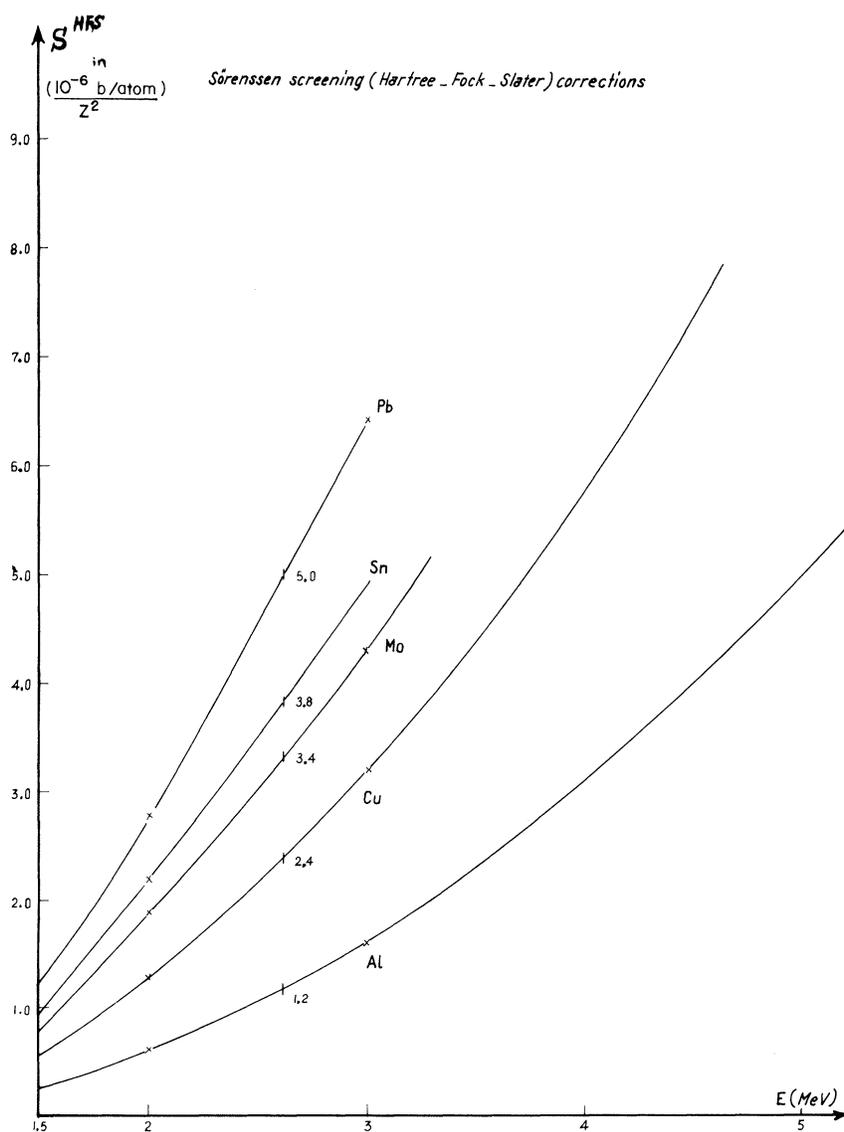
FIG. 7. Magnitude of Sørensen screening correction as a function of different material at a given energy.
