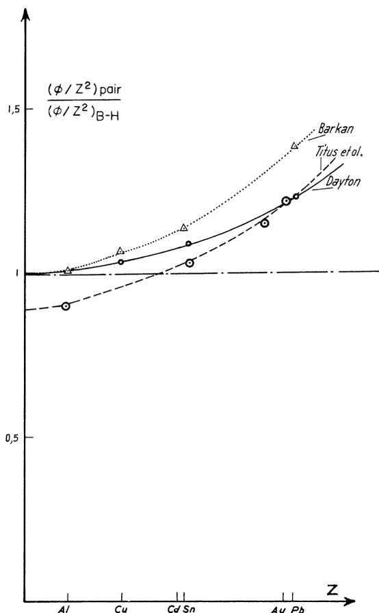
FIG. 3. Comparison of the relative cross sections measured by Titus *et al.*, Dayton, and the present author, in terms of Bethe-Heitler pair-production cross section calculated in the "exact Born" approximation.
