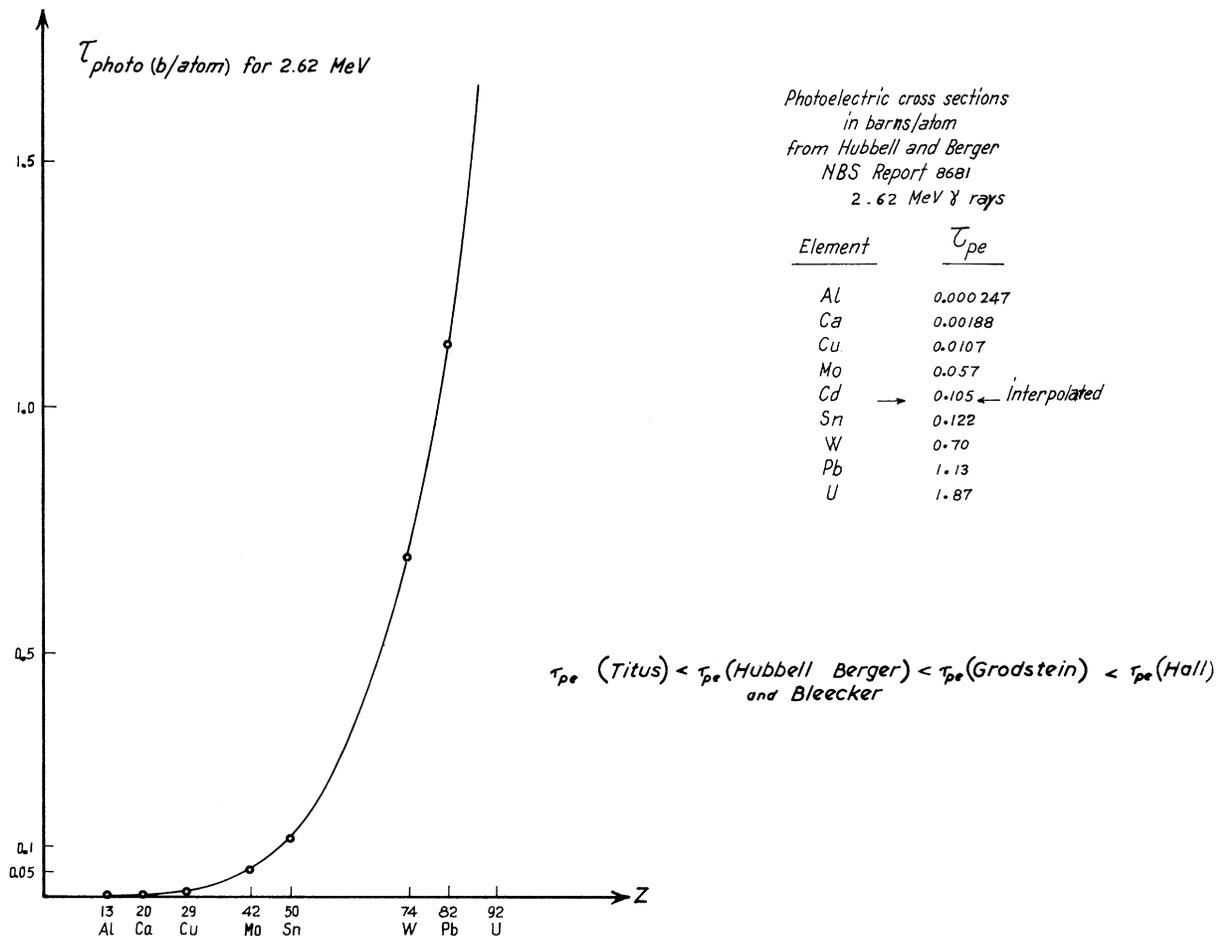
FIG. 1. Photoelectric cross section in b/atom as a function of atomic number  $Z$  for 2.62-MeV  $\gamma$ -ray energy according to the formula and other numerical data given by Hubbell and Berger.
