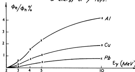
FIG. 5. Percentage decrease on total pair-production cross section due to triplet production, as a function of  $\gamma$ -ray energy in different material.
