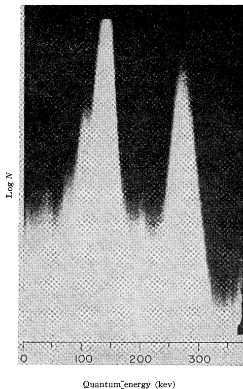
FIG. 6. Gray-wedge analyzer picture of \text{Se}^{75} gamma-ray spectrum (0 to 350 keV) as detected by a 3-cm diameter by 2-cm high \text{NaI}(\text{Tl}) crystal.
