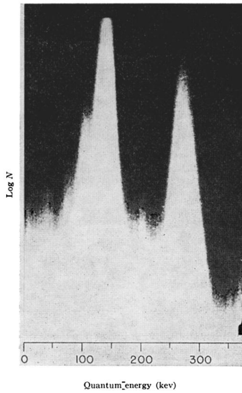
FIG. 6. Gray-wedge analyzer picture of ^{75}\text{Se} gamma-ray spectrum (0 to 350 kev) as detected by a 3-cm diameter by 2-cm high NaI(Tl) crystal.
