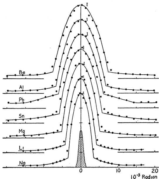
FIG. 1. The shaded curve is the calculated resolution. The central parabolas are computed from density, atomic weight, and valence, assuming an ideal Fermi gas at zero temperature. The abscissas of the sharp corners correspond to computed maximum momenta.
