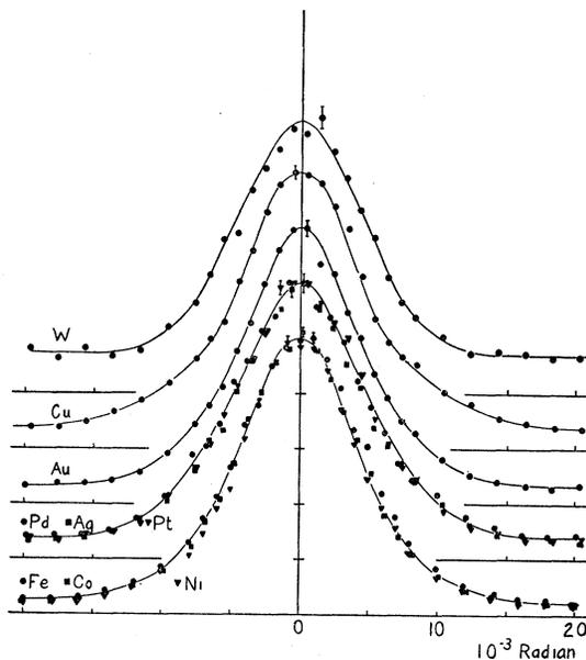
FIG. 3. Angular distributions from transition and noble metals. Curves are experimental.
