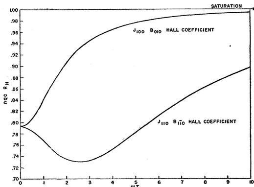
FIG. 1. Behavior of Hall coefficient plotted in terms of the universal parameter  $\omega\tau$  which simultaneously depicts the effect of magnetic field and scattering time: (a) The case  $\mathbf{J}_{100}, \mathbf{B}_{010}$ ; (b) the case  $\mathbf{J}_{110}, \mathbf{B}_{110}$ .
