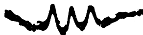
FIG. 3. Atomic N 14 hfs triplet. Broad-band oscilloscopic display and field modulation at 15 cps were used. The dissociator was an earlier Pyrex water-cooled version.
