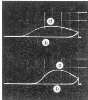
FIG. 4. Representative switching transients obtained by using a rectangular pulse of  $6\text{-}\mu\text{sec}$  duration of positive or negative sign and  $8.8\text{ kv/cm}$  amplitude: *a* indicates reversal, *b* nonreversal of polarization. Upper photograph taken at  $+23^\circ\text{C}$ , abscissa= $0.3\text{ }\mu\text{sec/div}$ ; lower photograph taken at  $-18^\circ\text{C}$ , abscissa= $0.1\text{ }\mu\text{sec/div}$ . Ordinate for both is  $=0.29\text{ amperes/division}$ .
