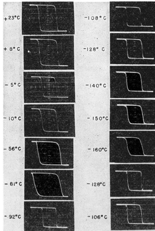
FIG. 1. Hysteresis loops as a function of temperature for the  $c$ -domain area of a  $\text{BaTiO}_3$  crystal. For all loops  $E=0.63$  kv/cm per horizontal division and  $Q=0.11 \times 10^{-6}$  coulomb per vertical division.
