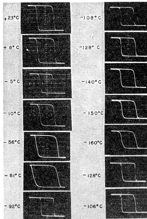
Fig. 1. Hysteresis loops as a function of temperature for the  $c$ -domain area of a  $\text{BaTiO}_3$  crystal. For all loops  $E=0.63 \text{ kv/cm}$  per horizontal division and  $Q=0.11 \times 10^{-6} \text{ coulomb}$  per vertical division.
