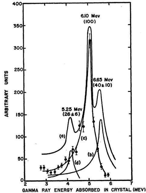
FIG. 3. Separation of high-energy spectrum of  $N^{14}(p,\gamma)O^{15}$  gamma rays into individual components. (a) Total curve. (b) 6.65-Mev line. (c) 6.10-Mev line. (d) 5.25-Mev line. Points and statistics are shown for the fluorine measurement.
