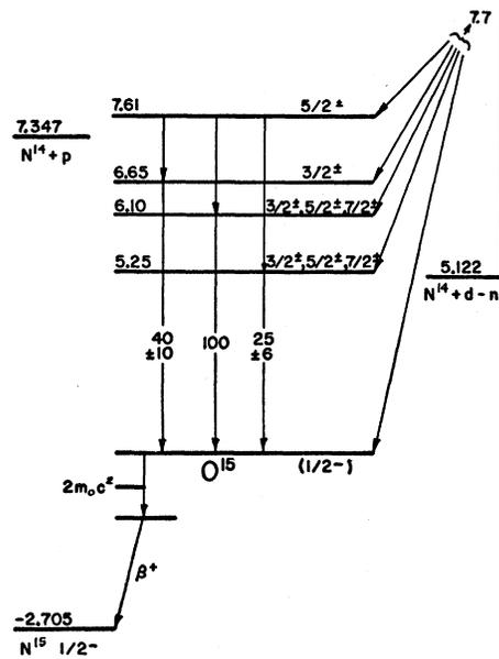
FIG. 5. Energy level diagram for O<sup>15</sup> for 7.61-Mev and lower states.
