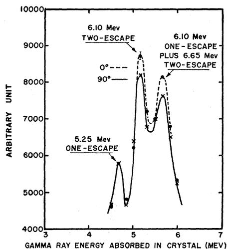
FIG. 4. Single-crystal spectra, at  $0^\circ$  and  $90^\circ$ , of high-energy gamma rays from 295-kev protons on thick TiN. Curves were normalized at 5.25-Mev one-escape peak.
