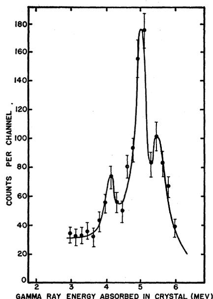
FIG. 2. Three-crystal, scintillation spectrometer analysis of gamma rays from  $N^{14}(p,\gamma)O^{15}$  reaction for 295-keV protons on thick TiN.
