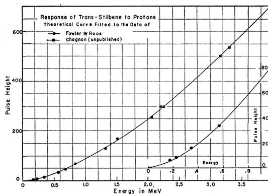
FIG. 6. Pulse heights *versus* proton energy for stilbene. Experimental data of Chagnon normalized to the curve at 3.3 Mev.
