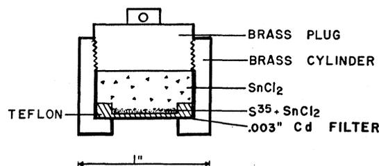
FIG. 1.  $S^{35}$ -Sn x-ray source used for calibrations.
