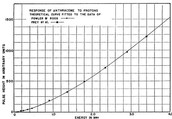
FIG. 5. Pulse heights *versus* proton energy for anthracene. Experimental data of Frey *et al.* (see reference 2) normalized to the curve at 3.4 Mev.
