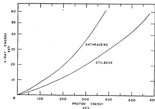
FIG. 4. X-ray energy *versus* proton energy for equal pulse heights.
