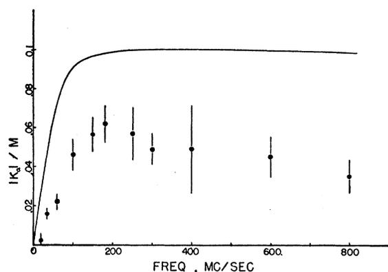
FIG. 4. Off-diagonal permeability component,  $|\kappa_a|$ , per unit magnetic moment vs frequency. Points are from present experiment on nickel ferrite, curve is from theory of domain rotation.
