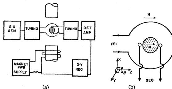
FIG. 1. (a) Block diagram of apparatus for observing domain rotation. (b) Diagrammatic sketch of rf head.
