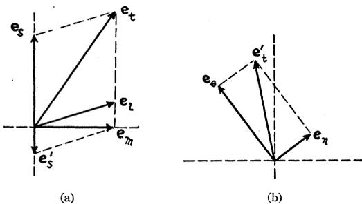
FIG. 2. Ac vector diagrams showing correction for effects of leakage signal. In (a) leakage is indicated by  $e_l$ , the desired precession signal by  $e_s$ , and the total observed signal by  $e_t$ . In (b)  $e_n$  is the residual leakage,  $e_\theta$  is the signal induced by loop angle deflection, and their result is shown as  $e_t'$ .
