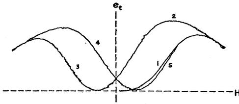
FIG. 3. Tracing from original  $x$ - $y$  recorder chart showing total output of magnetic induction apparatus for various applied steady fields extending into region of saturation. Starting from demagnetized state (origin) the branches were numbered in sequence as recorded.
