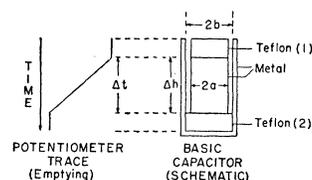
Fig. 1. Schematic representation of basic capacitor design and potentiometer record of emptying vessel by creep.
