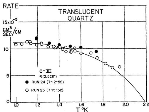
FIG. 6. Transport rates over translucent quartz specimen Q-III between 1.5 cm and 3.6 cm from the rim.
