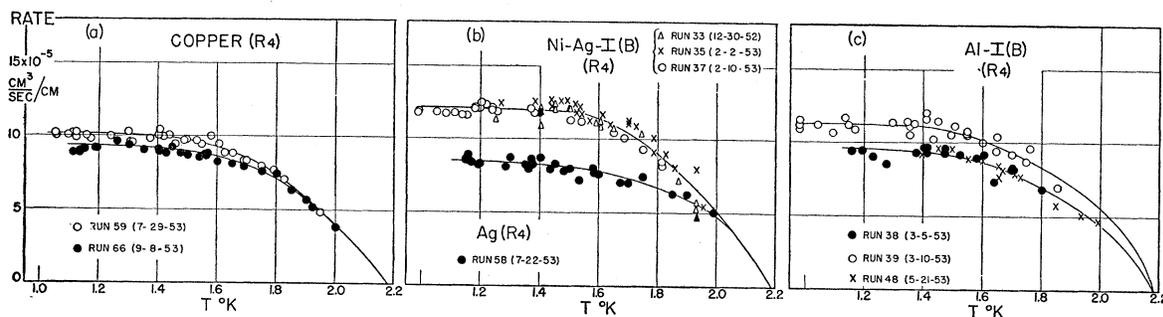
FIG. 8. Transport rates over various machined metal specimens: (a) copper, (b) nickel silver (upper curve), and silver (lower curve), (c) aluminum. In each case the transport rates were calculated for distances between 4.45 cm and 5.33 cm from the rim, corresponding to beaker region "4" in Fig. 2 and therefore designated as  $R_4$ .
