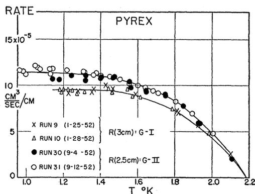
FIG. 4. Transport rates over Pyrex. Specimen G-I: averaged over distance from 1.9 cm to 4.1 cm from rim (lower curve); Specimen G-II: averaged over distance between 1.5 cm and 3.6 cm from rim (upper curve).
