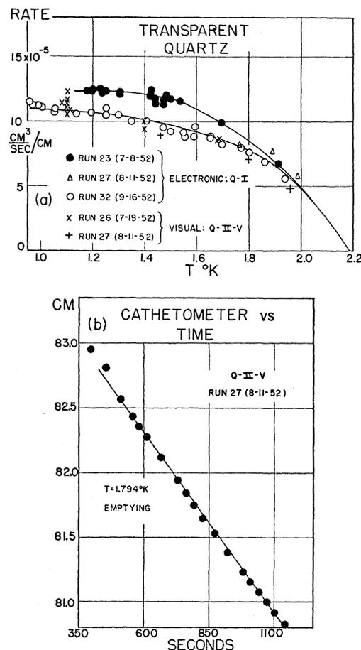
FIG. 5. (a) Transport rate over transparent quartz specimen Q-I, upper curve between 1.9 cm and 2.7 cm from the rim, lower curve between 1.5 cm and 3.6 cm from the rim. (b) Typical record of visual observation of rate of fall of helium meniscus in quartz capillary used in calculating rates shown in (a) for specimen Q-II-V.
