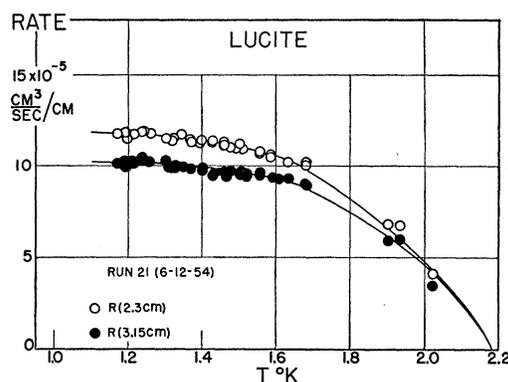
FIG. 7. Transport rates over Lucite, averaged between 1.9 cm and 2.7 cm from the rim (upper curve) and between 2.8 cm and 3.6 cm from the rim (lower curve).
