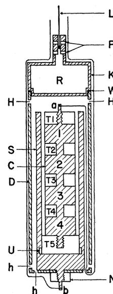
FIG. 2. Cross section of typical transport vessel-capacitor assembly in radiation shield (not to scale).
