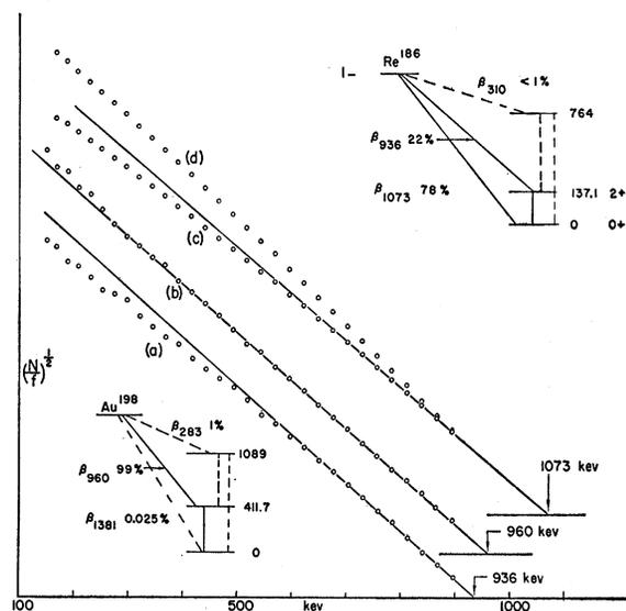
FIG. 1. Kurie plots of: (a)  $\text{Re}^{186}$  coincidence spectrum; (b)  $\text{Au}^{198}$  coincidence spectrum; (c)  $\text{Re}^{186}$  ground-state transition by subtraction; (d)  $\text{Re}^{186}$  total singles spectrum.
