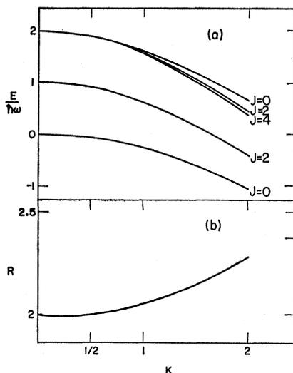
FIG. 3. (a) The energy levels as a function of the coupling strength  $K$ .  $K=0.67[(\hbar^2/2B)/\hbar\omega]^{1/2}k$ , where  $B$  denotes the mass parameter and  $k$  the coupling parameter. (b)  $R=E_2/E_1$ , where  $E_1, E_2$  denote the energy above the ground state of the first and second  $2+$  state respectively. The anharmonic terms are not included.
