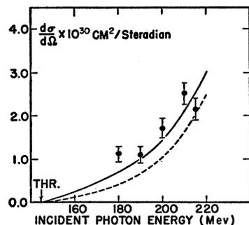
FIG. 2. Differential cross sections at  $135^\circ$  in the center-of-mass system versus laboratory photon energies. For discussion of curves see text.
