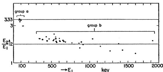
FIG. 2. Ratio of energies  $E_2/E_1$  as function of  $E_1$  for  $36 \leq N \leq 108$ . The character of the second excited state of the even-even nucleus is denoted by  $\blacktriangle$  ( $0+$ ),  $\blacksquare$  ( $2+$ ),  $\times$  ( $4+$ ), and  $\bullet$  (not known). Points for nuclei with odd spin for the second excited state are omitted from this figure.
