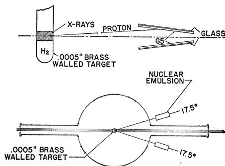
FIG. 1. Schematic diagram of liquid target and nuclear emulsion detectors.
