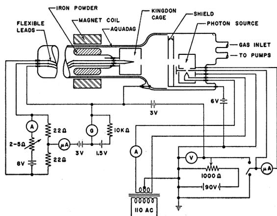
FIG. 1. Cross section of experimental tube with circuit diagram.
