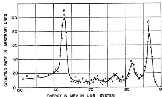
FIG. 1. Scattering from a  $\text{CH}_2$  target at  $80^\circ$ . The C and H peaks are due to electrons scattered elastically from carbon and hydrogen, respectively. The remaining peaks are due to electrons scattered inelastically from carbon.
