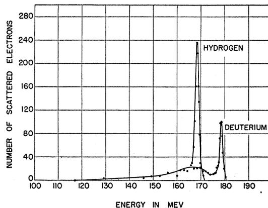
FIG. 5. Scattering from hydrogen and deuterium at 70° using gas targets.
