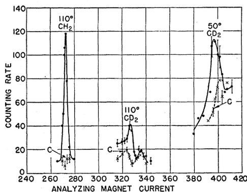
FIG. 2. Scattering from  $\text{CH}_2$  and  $\text{CD}_2$  targets at  $110^\circ$  and  $50^\circ$ . Scattering from a pure-carbon target is also shown. The ordinate scale for the two angles shown is different for each. Uncertainties shown for the ordinates are due to counting statistics alone.
