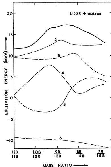
FIG. 1. Excitation energy as a function of mass splitting for thermal fission of  $U^{235}$ . Curve 1: Excitation energy  $E$  of the fragment pair; it is the sum of the five components 2 to 6. Curves 2,3: Mass corrections  $\Delta M_A$  for heavy and light fragments respectively. Curves 4,5: Contributions due to the corrections  $\Delta Z_A$  for heavy and light fragments respectively. Curve 6: Excitation energy  $E$  of the fragment pair using uncorrected semiempirical mass formula.
