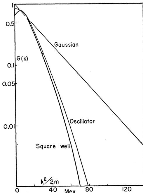
FIG. 1. Momentum distribution  $G(k)$  of 8 neutrons and 8 protons in the independent-particle states of a square well with infinite walls and of a harmonic oscillator well. For comparison the Gaussian distribution of Eq. (3) is also given.
