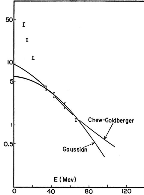
FIG. 2. Theoretical predictions for the photoproton process based on a Chew-Goldberger and on the Gaussian distribution of Eq. (3). The experimental data are taken from the paper of Levinthal and Silverman (see reference 7). The theoretical results are normalized to the experiments at 41.5 Mev by a factor of 0.75 for the Chew-Goldberger and 0.15 for the Gaussian.
