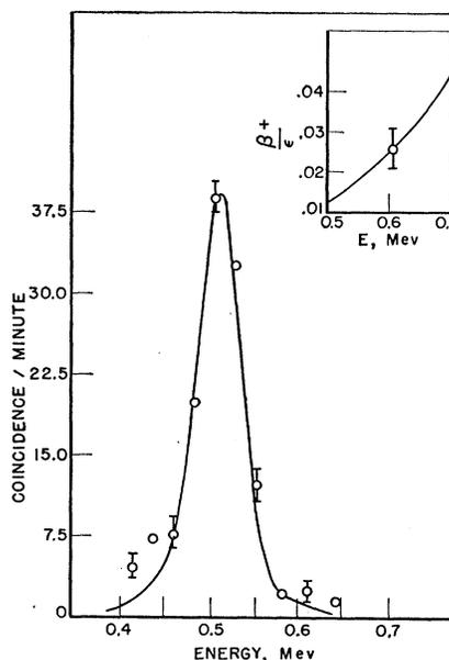
Fig. 4. Spectrum of  $\gamma$  rays in coincidence with the 0.161-Mev  $\gamma$  in the decay of  $\text{Sb}^{117}$ . The solid curve is the  $\text{Na}^{22}$  annihilation radiation energy calibration. The insert is a graph of the theoretical  $\beta^+/\epsilon$  ratio for Sb with the experimentally measured ratio shown as a point.
