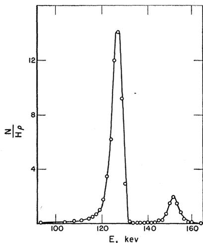
Fig. 3. Conversion electron spectrum of the 0.161-Mev  $\gamma$  of  $\text{Sb}^{117}$ .
