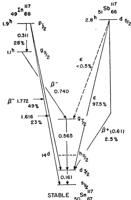
FIG. 5. Decay scheme for  $\text{In}^{117}$  and  $\text{Sb}^{117}$ .
