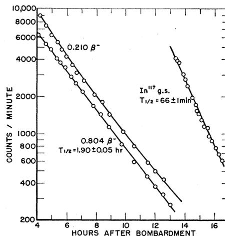
FIG. 1. Decay curves of 0.210- and 0.804-Mev betas of  $\text{In}^{117m}$  as measured with the lens spectrometer and the decay curve of the 0.161-Mev  $\gamma$  of the  $\text{In}^{117}$  ground state.
