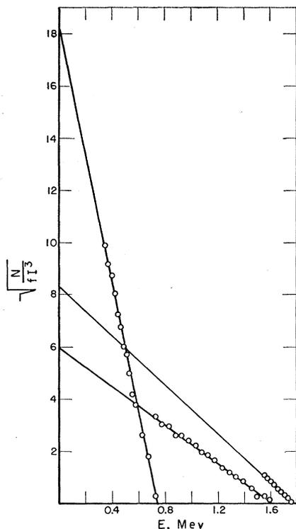
Fig. 2. Fermi-Kurie plot of the  $\text{In}^{117}$  beta spectra showing the end points of 1.772, 1.616 and 0.740 Mev.
