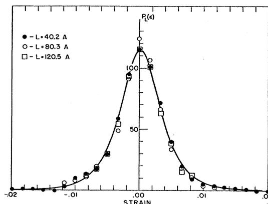
FIG. 2. Points from the synthesized strain distributions for  $L=40.2$  A, 80.3 A, and 120.5 A in a single crystal of LiF irradiated  $7.5 \times 10^{17}$  nvt, and the function  $P_L(\epsilon) = (\frac{1}{3}\sigma) [\cosh\pi(\epsilon - \bar{\epsilon})/2\sigma]^{-1}$  with  $\bar{\epsilon} = 0.00012$  and  $\sigma = 0.00438$ .
