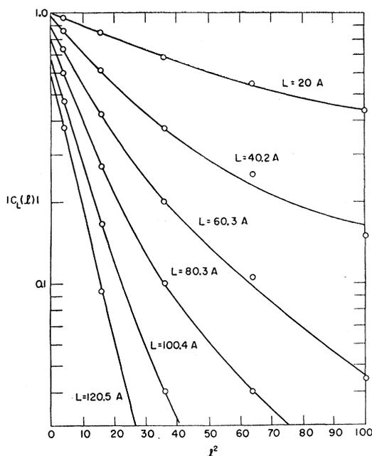
FIG. 1. Semi-log plot of  $|C_L(l)|$  versus  $l^2$  for the first five orders of (00 $l$ ), measured on a single crystal of LiF irradiated  $7.5 \times 10^{17}$  nvt.
