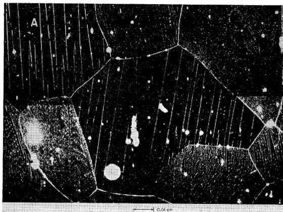
FIG. 1. Domains of reverse magnetization on well-oriented material, showing that in the demagnetized state these domains are not influenced by the orientation of the adjacent grains.
