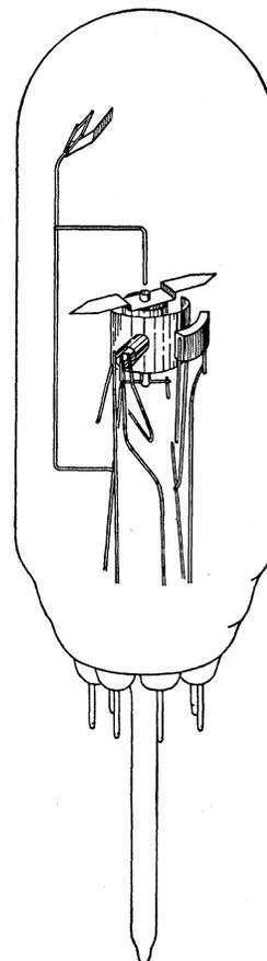
FIG. 1. Structure of vacuum tube utilized in determining electron energies and surface potentials.
