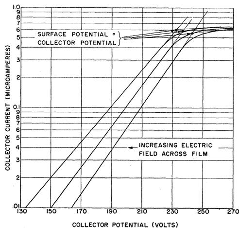
FIG. 3. Collector current as a function of collector potential. The variation of electron energies and surface potentials as a function of the electric field are also illustrated.
