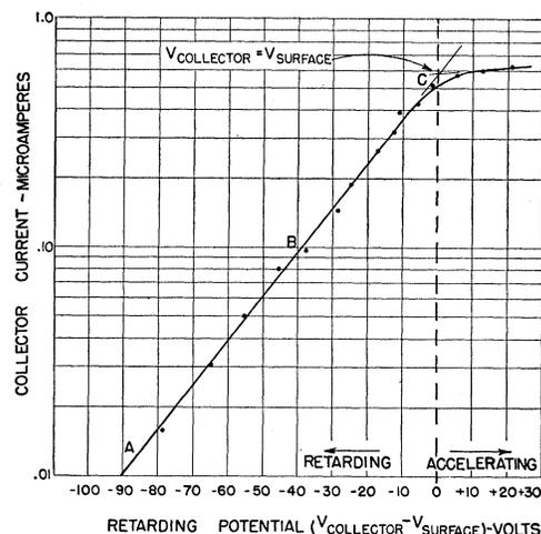
FIG. 4. Collector current as a function of retarding potential (dynode potential 100 volts and surface potential 226 volts), assuming the knee of the curve to represent zero surface potential.
