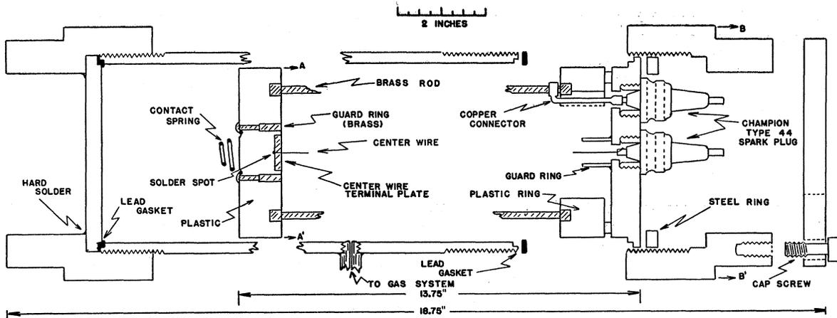
FIG. 1. Schematic drawing of high-pressure proportional counter.
