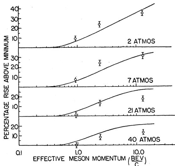
FIG. 7. Comparison of the theoretical rise of the most probable ionization energy loss (based on Sternheimer's calculations for the density effect) with the observed value at various gas pressures.
