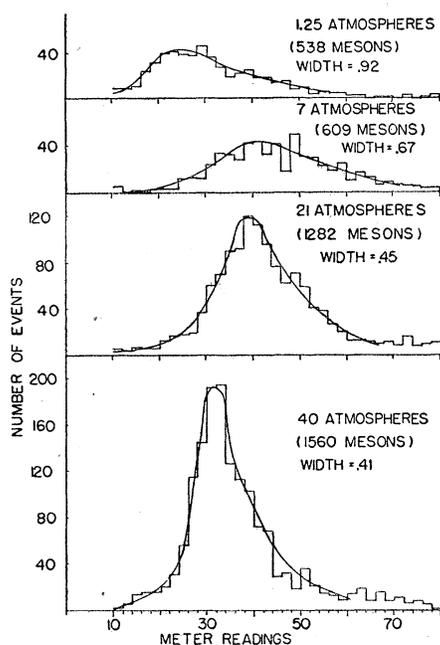
FIG. 4. Combined histograms for entire meson spectrum for various gas pressures in the high-pressure proportional counter.
