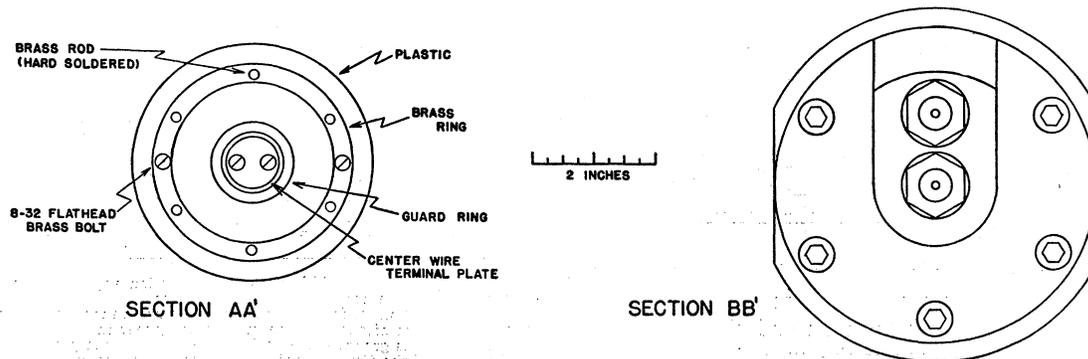
FIG. 2. Cross sections of high-pressure proportional counter.
