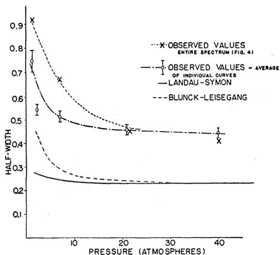
FIG. 5. Comparison of the theoretical and observed values of the width at half-maximum of the Landau distribution as a function of gas pressure.
