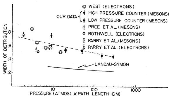
FIG. 6. Comparison of theoretical and all observed values of the width at half-maximum of the Landau distribution as a function of the logarithm of the amount of material traversed.
