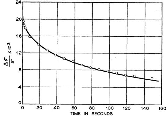
FIG. 7. The decay in photoconductivity as a function of time caused by the deep traps in *p*-type Si 223B. The ordinate is the fractional change in conductivity, and zero time on the abscissa is the instant the light is removed from the specimen. The open circles are experimental points, and the solid line is a fit of Eq. (10), Appendix, to these points. The values of the parameters in the equation that are determined by the fit are given in the text.
