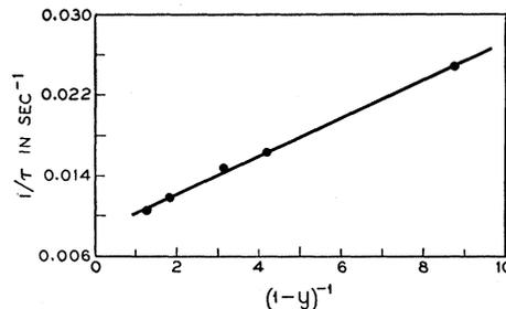
FIG. 11. Replot of the data, Fig. 10, as suggested by Eq. (31) which is derived on the assumption that, in addition to simple multiple-trapping, recombination in the trap also occurs.
