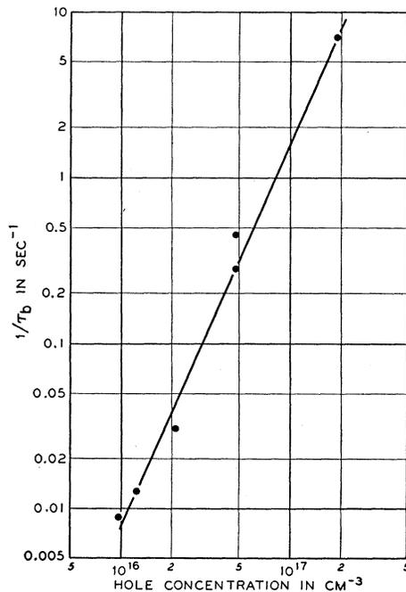
FIG. 12. Plot of the rate of recombination in the deep traps,  $1/\tau_b$ , as a function of the majority carrier concentration. Within the experimental error, the slope of the line equals 2.
