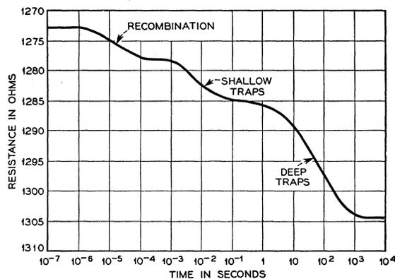
FIG. 4. Change with time of the resistance of *p*-type Si rod 223-B after a strong light has been removed from the specimen. The photoconductivity of the rod decays in three well-defined steps, the first (in sequence of time) is attributed to recombination of electrons in the conduction band; the second is attributed to the emptying of shallow traps; and the third is attributed to the emptying of deep traps.
