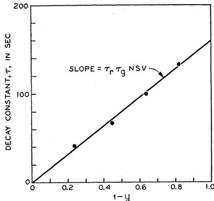
FIG. 9. Plot of the apparent time constant  $\tau$  as a function of  $(1-y)$ , the fraction of deep traps empty (specimen VI-550-1,  $\rho = 17$  ohm cm). According to the simple multiple-trapping model Eq. (13), this plot should be a straight line with intercept at  $y \equiv n_2/N = 1$  equal to  $\tau_g$ . The quantity  $\tau_g$  is too small to be resolved on this time scale.
