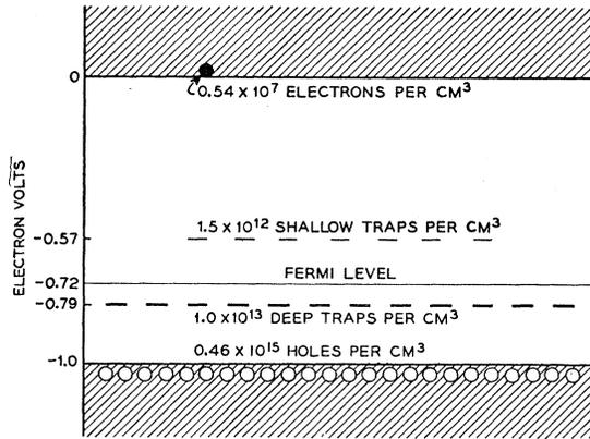
FIG. 8. Diagram depicting the number and relative energy of the traps for electrons in *p*-type Si 223B. Zero of energy is the bottom of the conduction band. The numbers given were computed assuming the specimen to be at room temperature.
