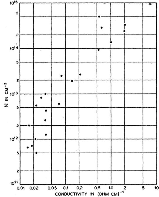
FIG. 13. Plot of the number of empty (deep) traps vs sample conductivity showing a rough correlation which can be accounted for largely by the position of the Fermi level if the number of trapping centers in each specimen is roughly constant.
