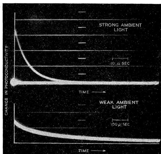
Fig. 3. Photographs of the oscilloscope trace in the experiment shown in Fig. 2. Top—with strong ambient light falling on a *p*-type silicon specimen, no trapping is observed and the decay in photoconductivity as a function of time represents the true lifetime of the added electrons. Bottom—without ambient light trapping occurs, and it controls the decay in photoconductivity.
