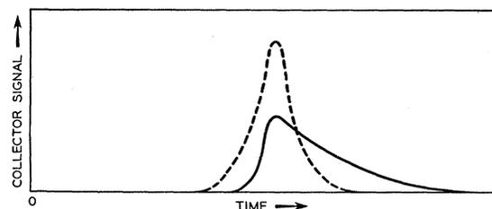
FIG. 1. Collector signal (schematic) as a function of time in the drift mobility experiment. The broken line is typical of Ge at room temperature regardless of ambient light and of Si at room temperature in strong ambient light. The solid line is typical of *p*-type Si in weak ambient light when some trapping of minority carriers occurs.
