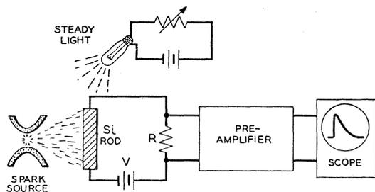
Fig. 2. Schematic diagram of circuit used to measure the lifetime of minority carriers and to study the trapping of minority carriers.
