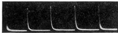
FIG. 10 Streamers in oxygen, 300 mm Hg, 3050 volts, 1000 \mu sec full scale, RC=3 \mu sec. Single sweep—gain 1/200 that on Fig. 9.
