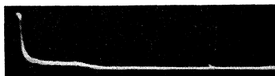
FIG. 8. Ion drift pulse in oxygen with amplification but with no secondary action, 300 mm Hg, 2775 volts, 1000 \mu sec full scale, RC = 3 \mu sec.
