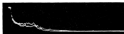
FIG. 9. Burst pulses in oxygen, 300 mm Hg, 2900 volts, 1000 \mu sec full scale, RC = 3 \mu sec. Single sweep.
