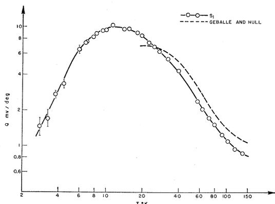
FIG. 1. Thermoelectric power of *p*-type germanium samples.
