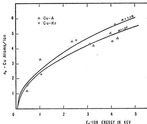
FIG. 3. Copper-krypton and copper-argon sputtering ratios vs ion energy.
