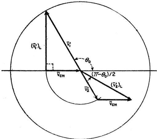
FIG. 5. Collision diagram. Subscript  $L$  denotes velocity in the laboratory frame. Primes denote velocity after collision. Subscript 1 or 2 denotes gas or metal atom velocity.
