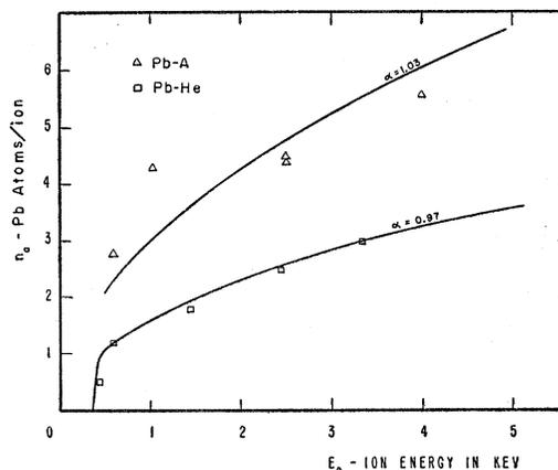
FIG. 4. Lead-argon and lead-helium sputtering ratios vs ion energy.
