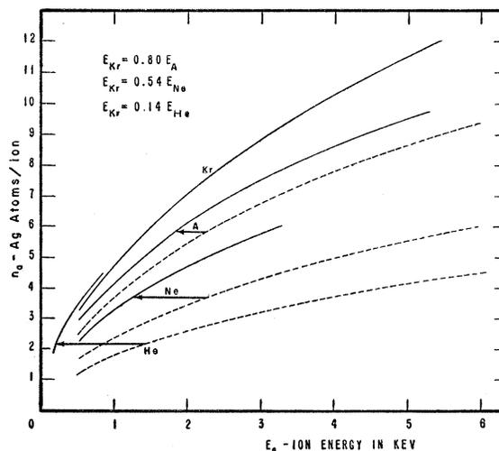
FIG. 7. Equivalent energy shift of helium, neon and argon sputtering ratio curves relative to krypton on silver.
