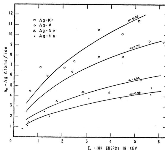
FIG. 2. Silver series of sputtering ratio vs ion energy for Ag-Kr, Ag-A, Ag-Ne, Ag-He.
