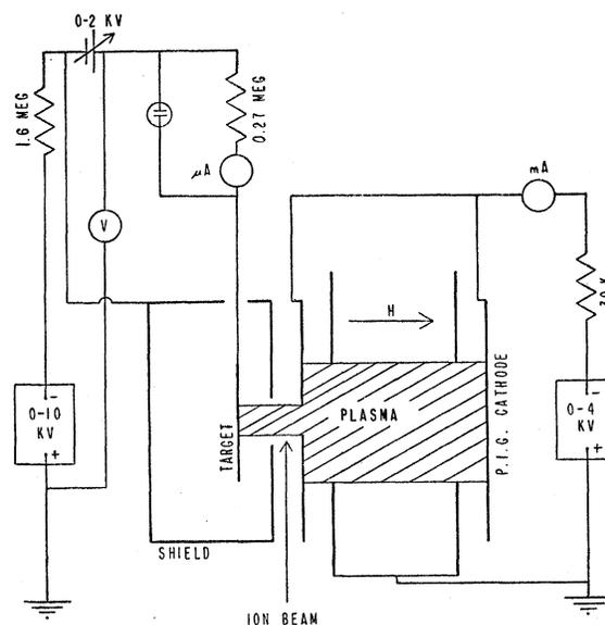
FIG. 1. The ion beam electrical circuit.
