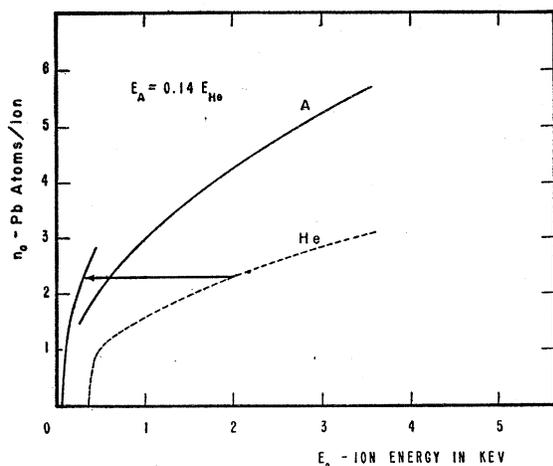
FIG. 6. Equivalent energy shift of helium sputtering ratio curve relative to argon on lead.
