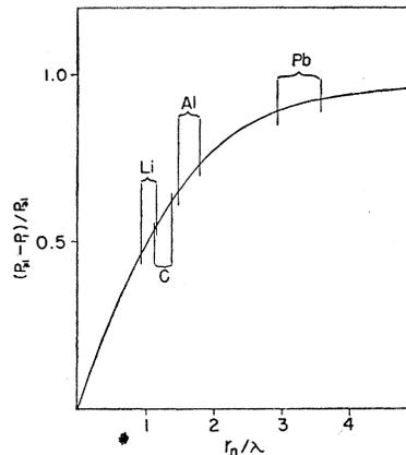
FIG. 5.  $(P_{\geq 1} - P_1)/P_{\geq 1}$ , the fraction of events in which the primary undergoes more than one collision, as a function of  $r_n/\lambda$ .
