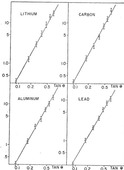
FIG. 4. "F plots":  $\log(F/1-F)$  vs  $\log(\tan \theta)$ , for all four elements.
