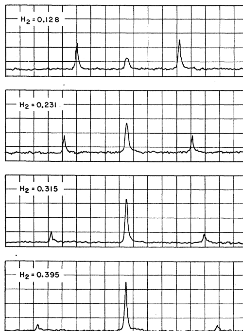
FIG. 4. Effect on the fluorine spectrum of varying the phosphorous rf amplitude H_2 , with \omega_2 = \gamma_2 H_0 . The top and bottom traces of Fig. 2 are also part of this series.
